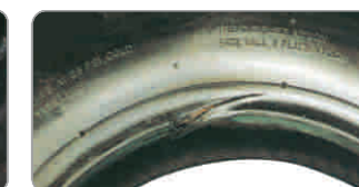
Tire lip lesion (Machinery installation tires) Improper operation when tires and rims assembly, Causing tire labial ministry damage by tires machine, unloading tires machine
