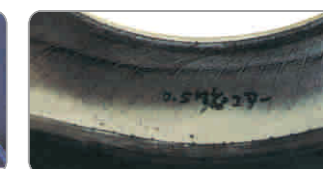
Wrapped drape inside Tires run with low air pressure, causing tire body buckling and chicken claw marks on inside face.
