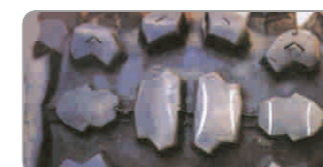
Tread bottom cracking Tires running with low air pressure long time, killing tread bottom
