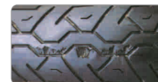
Tire surface damage Tires stuck sharp objects, do strong traction action and damage. Commonly occurring in the back tire.
