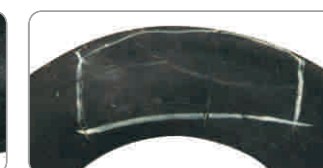
Sandwiched eyewinker When assembly tire, there's sandwiched eyewinker between inner tubes and tires which not been clear, causing damages on tire and inner tube.
