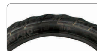
Abnormal abrasions (polygonal) Faults on vehicle parts, cause tires polygonal abrasion.
