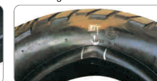
Tire lip wire break When tire and tire rims engage with discomfort state, tire was forced by high-pressure air injected, causing stress concentration in discomfort joint place ,making wire at tire lip broke.
